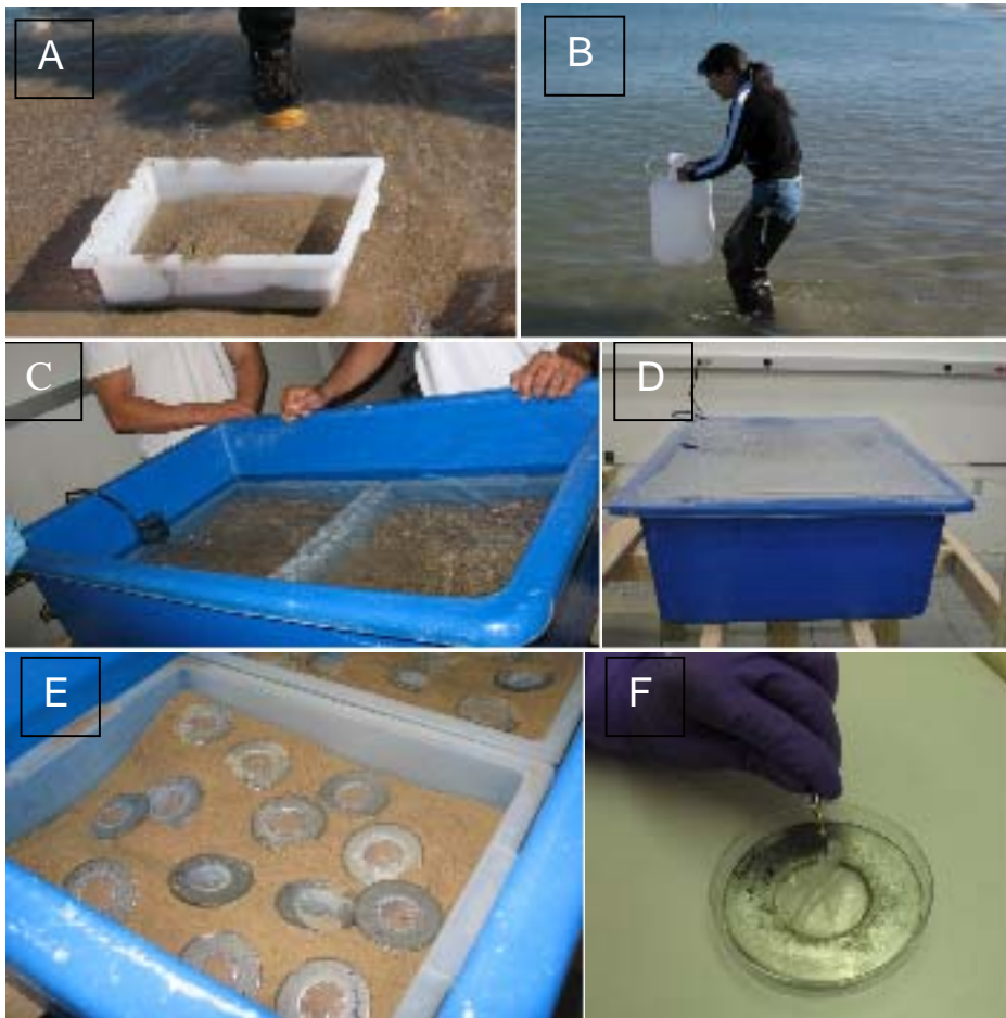
Figure 1 Set up of diffusion chambers and simulated natural environment. (A) Field collection of sediment. (B) Field collection of water using 25L carboys. (C and D) Simulated natural environment set up in laboratory using collected Lake Michigan sediment and water. (E) Diffusion chambers incubated on the surface of the sediment. (F) Diffusion chamber being opened for observation after incubation in the simulated natural environment.
